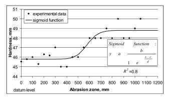
**Figure 5.** Change of frame saw blade side plane hardness upwards to the top end (sigmoid function coefficients: a=45.7765; b=3.0248; c=578.9751; d=47.5412)
