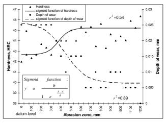
**Figure 7.** Interrelations of hardness-wear on saw blade side plates within abrasion zone (hardness sigmoid function coefficients: a=42.6530; b=2.5587; c=372.5658; d=55.2834; depth of wear sigmoid function coefficients: a=0.00643; b=0.0194; c=438.6372; d=-106.8771)
