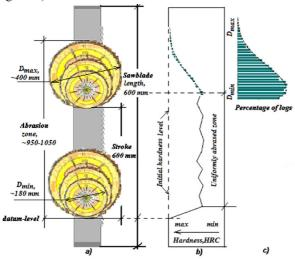
**Figure 1.** Modelling of saw blade abrasion in the kerf within logs contact zone during one frame stroke: a)-location of logs  $D_{min}$ - $D_{max}$  at the upper and lower dead-points of the saw blade stroke; b)-uniformly abraded zone; c)-typical sawlog size distribution
