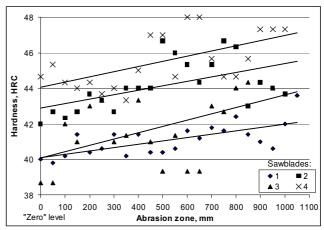
Figure 6. Change of surface hardness within abrasion zone of four tested saw blades
