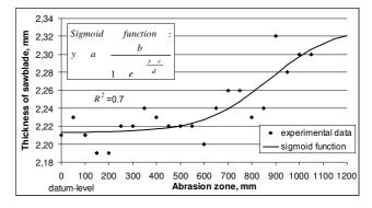
**Figure 4.** Change of frame saw blade thickness upwards to the top end (sigmoid function coefficients: a=2.2129; b=0.1182; c=872.677; d=138.8371)
