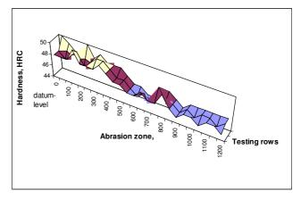
Figure 3. Typical pattern of surface hardness on used frame saw side plane
